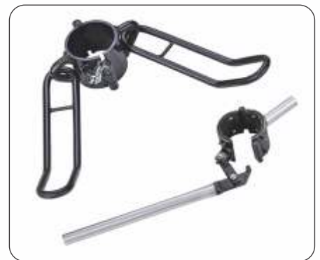
Sigri (Pipe lifting) Spanner (Pipe tightening)
