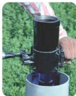
Fix bottom adapter with pump
